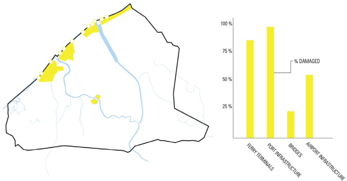
Figure 7.4. Damage Distribution - Transportation
